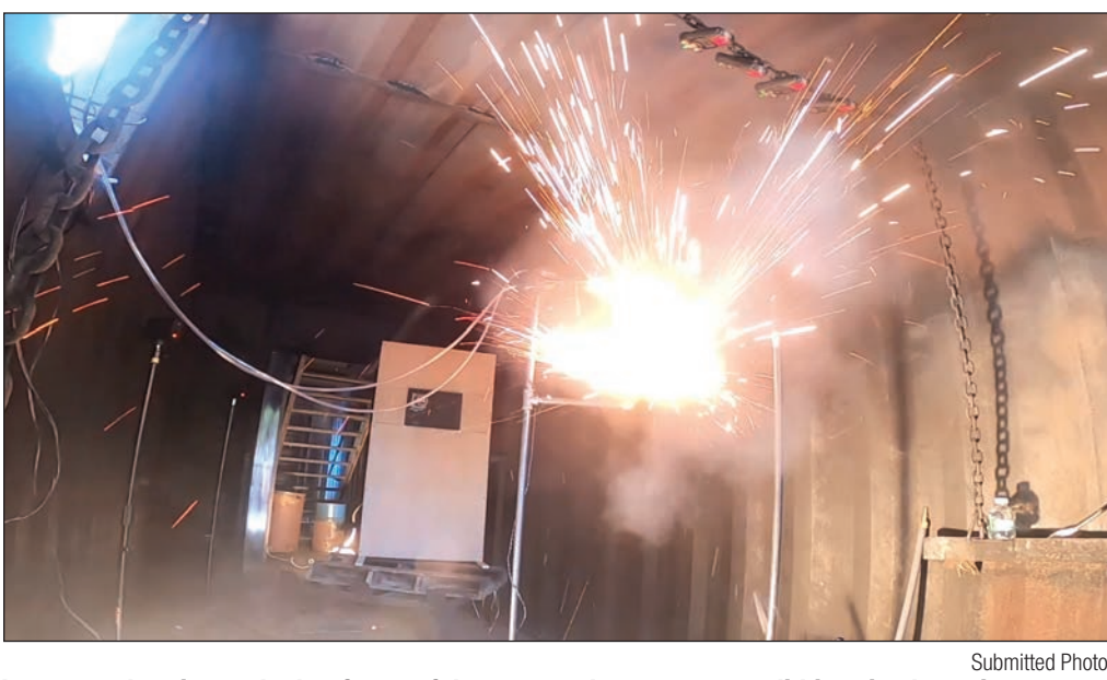
Submitted Photo Improper charging and other forms of damage or abuse can cause lithium-ion batteries to ignite, causing a fire. This battery, identical to the ones used in many consumer devices, exploded under controlled conditions during a 2023 research event held by the Department of Fire Services, New Bedford Fire Department, and other partners.
